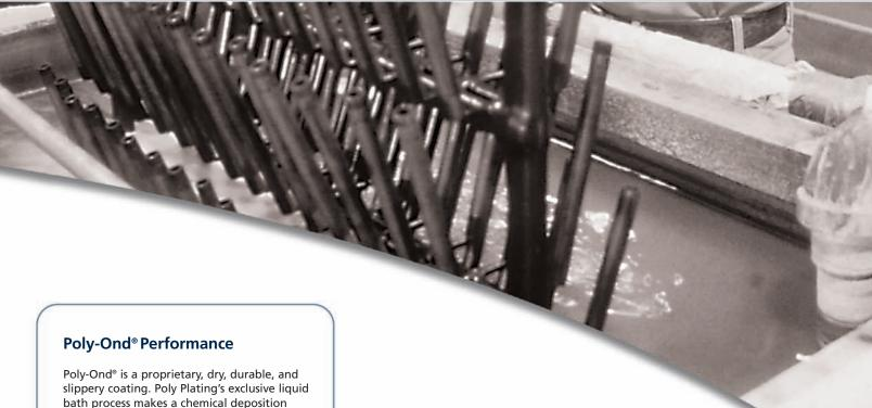
Poly-Ond® is a proprietary, dry, durable, and slippery coating. Poly Plating's exclusive liquid bath process makes a chemical deposition of nickel and phosphorus, impregnated with polymers, on the surface of metals. The result is a range of unique performance properties unmatched by any other metal plating technology.
